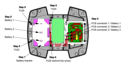
Figure 12: Installing G-1 Beam batteries IV
