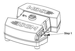
Figure 9: Installing G-1 Beam batteries I
