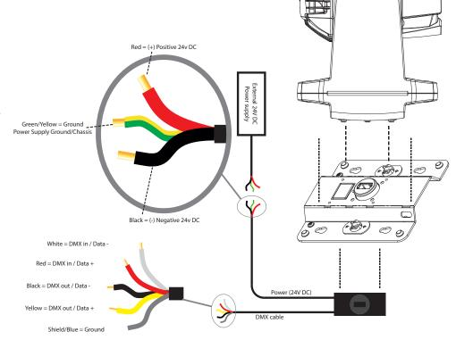
Figure 20: Connecting ceiling mount bracket to DC and DMX
