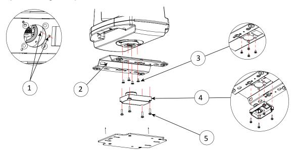
Figure 18: Attaching the ceiling mount bracket
