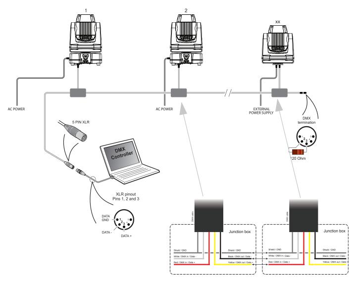
Figure 28: Connecting DMX and AC Power in G-1 Beam POI
