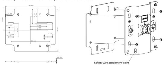
Figure 19: Installing the ceiling mount bracket
