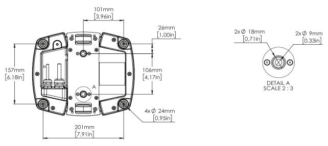
Figure 25: G-1 Beam POI base with dimensions
