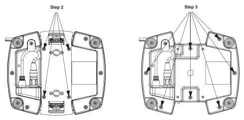
Figure 10: Installing G-1 Beam batteries II
