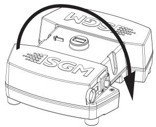
Figure 11: Installing G-1 Beam batteries III
