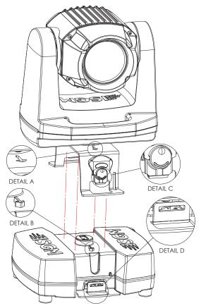
Figure 16: Removing G-1 Beam head
